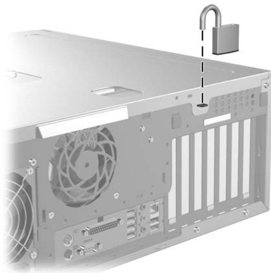
Figure 4-3 Removing the security lock
