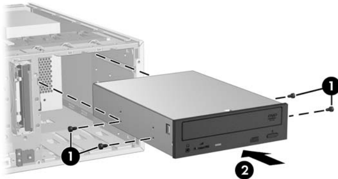
Figure 4-39 Installing the optical drive
