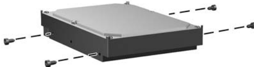
Figure 4-46 Installing hard drive installation guide screws
