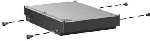
Figure 4-45 Removing hard drive installation guide screws
