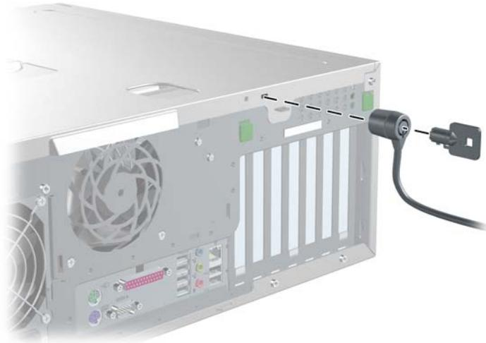
**Figure 4-5** Removing the cable lock
