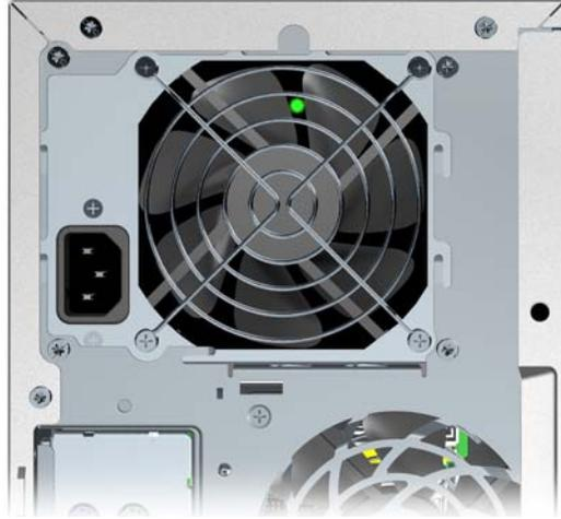
**Figure 5-1** Testing power supply with BIST LED
