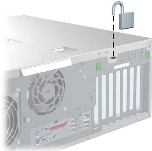
**Figure 4-4** Removing the security lock
