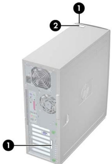
**Figure 1-4** Serial number and COA label location
