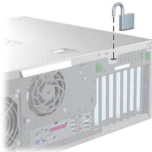
**Figure 4-4** Removing the security lock
