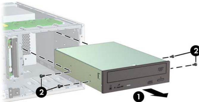
**Figure 4-38** Removing the optical drive screws
