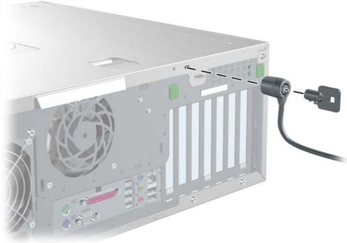
**Figure 4-5** Removing the cable lock
