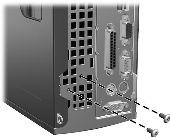
2. Remove the workstation access panel (Section 5.5).
