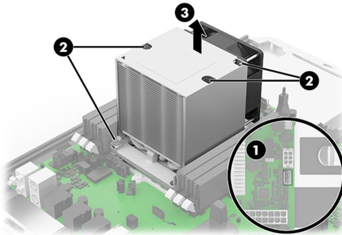
Reverse this procedure to install the heat sink.
