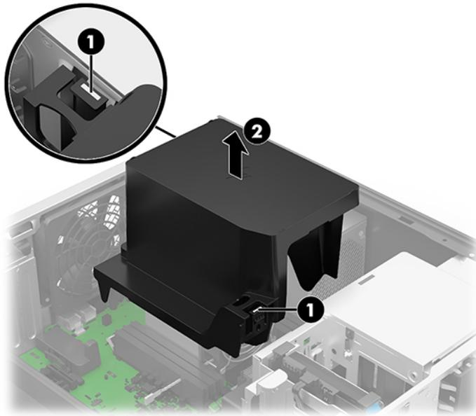
Reverse this procedure to install the memory fan.
