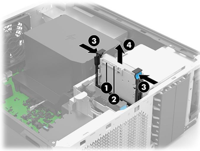
6. Separate the drive cage retention arms **(1)** from the storage device, making sure the retention pins **(2)** fully release from the device.
