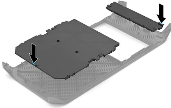
5. Align the outer bezel with the chassis and move it closer until it attaches magnetically.
