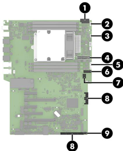
3. Remove the nine Torx15 M3.0×6.0 screws (1) that secure the system board to the computer.
