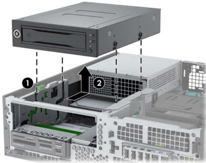
8. If you are replacing the DX115 unit, remove and retain the four M3 x 5mm screws (black) from the lower four mounting holes of the DX115 case, and then transfer the screws to the new unit. (You can also store the screws in the chassis. See [Locating extra guide screws on page 72](#) for screw locations.)
