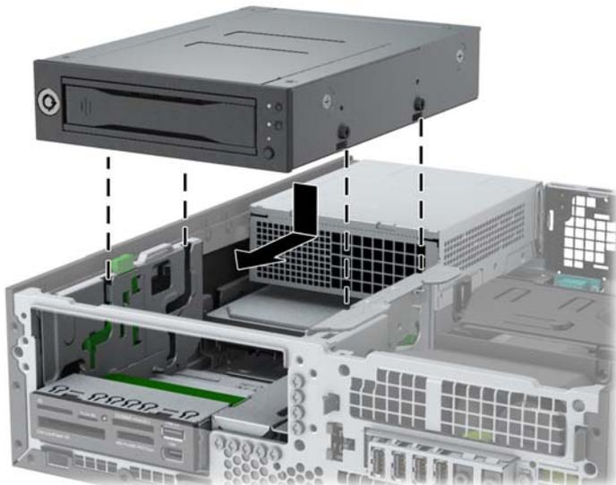
6. Rotate the drive cage to its upright position.
