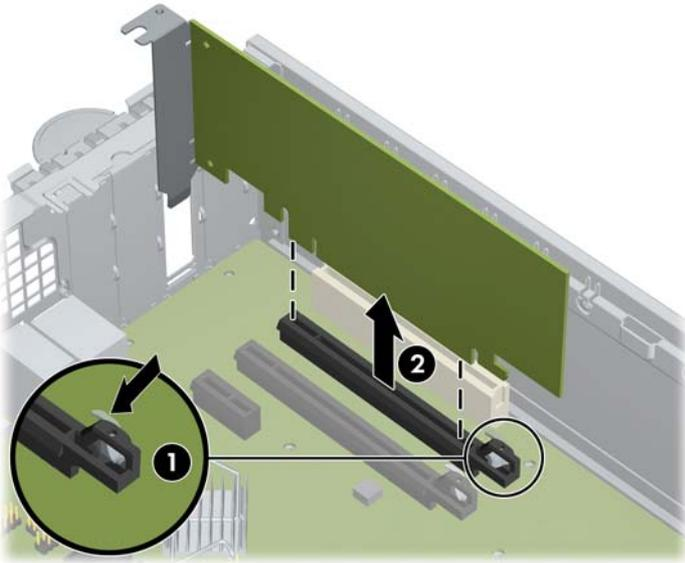
6. Push the retention latch and install an expansion slot cover if you do not intend to replace the card.
