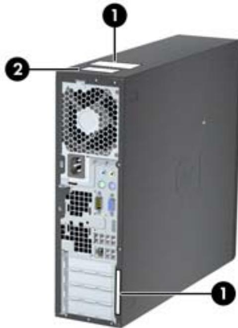
In general, the serial number labels can be found on the top panel or on the side of the computer and at the rear of the computer (your computer may look different). Keep this number available when contacting customer service for assistance.
