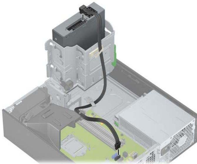
8. Connect the power cable (1) and data cable (2) to the rear of the DX115 case.
