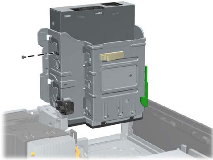
6. Carefully rotate the drive cage back down to its normal position.
