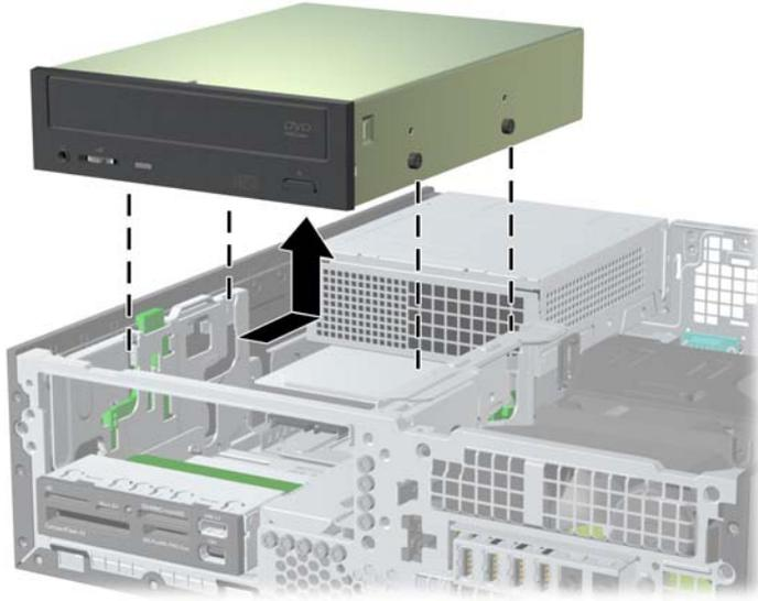
8. If you are replacing the drive, transfer the four guide screws from the old drive to the new one.
