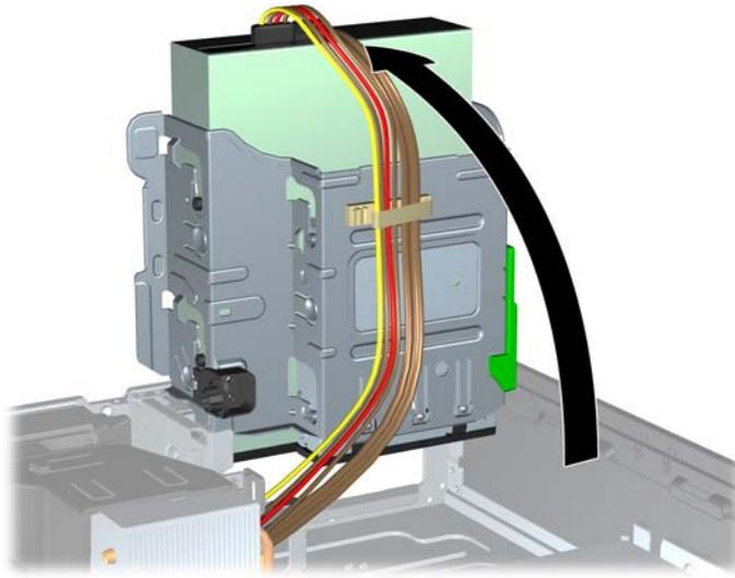
5. Carefully guide the front panel I/O device assembly cables through the chassis openings from which they were removed.
