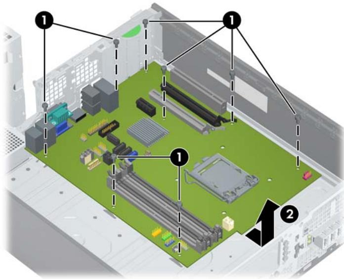
9. Lift the system board slightly, and pull the board away from the rear of the chassis.
