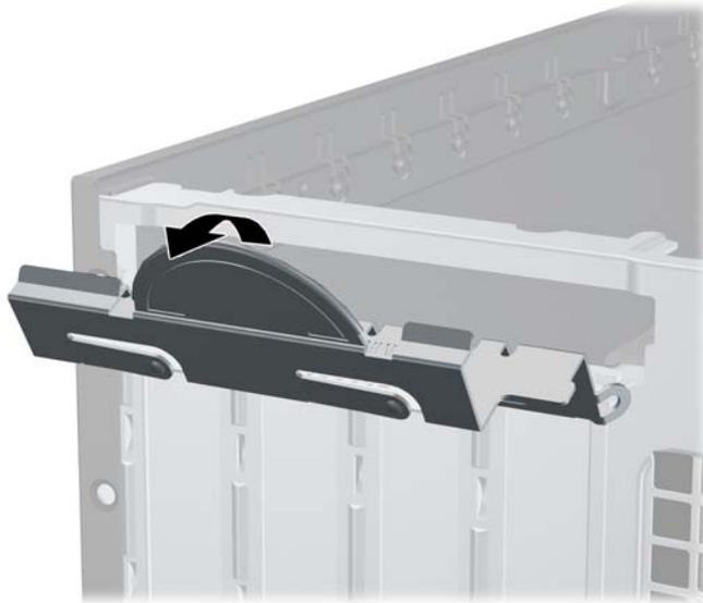
5. If the card slot has a latch, release the latch (1), and then carefully lift the card from the chassis (2).
