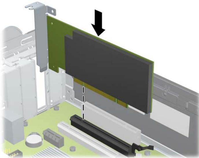
7. Close the expansion card retention clamp by rotating it downward.
