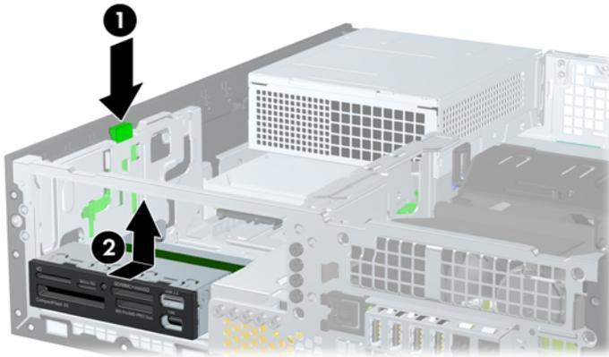
7. Rotate the drive cage back down to its normal position.
