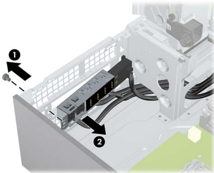
6. Disconnect the front panel I/O device assembly cables from the system board as shown below.
